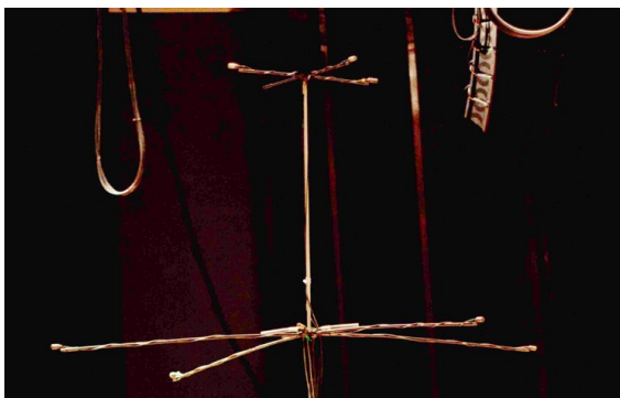
FIGURE 5 – MAGIC ARRAY + 2 ND LAYER ARRAY FOR ELEVATION
