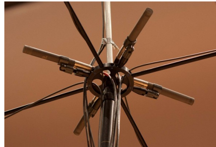
FIGURE 6 – THE ‘WILLIAMS HYPOCARDIOID CROSS’ - CENTRE OF THE HUB OF THE MAGIC ARRAY -
