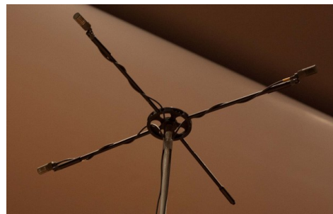
FIGURE 8 – 2 ND LAYER (3 MICROPHONES) SUPERCARDIOID ELEVATION ARRAY
